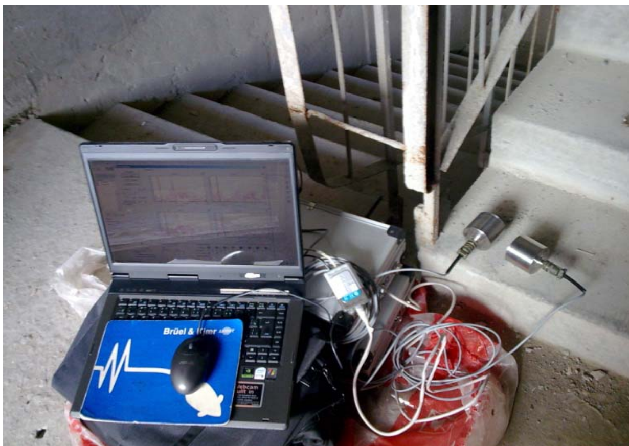
Mobile device for measuring ground and building structures vibration
